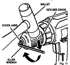
Open chuck jaws and remove allen wrench. Remove the chuck screw by turning it in a clockwise direction. See Figure 12. Note: The screw has left hand threads.
